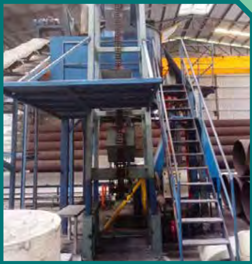
Bituman Charging Covenyor for cement lining pipe process, operational improvement.
