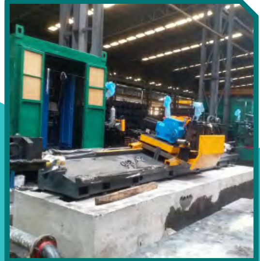
New Cold Saw Machine to replace conventional friction saw fly cutter, operational improvement.
