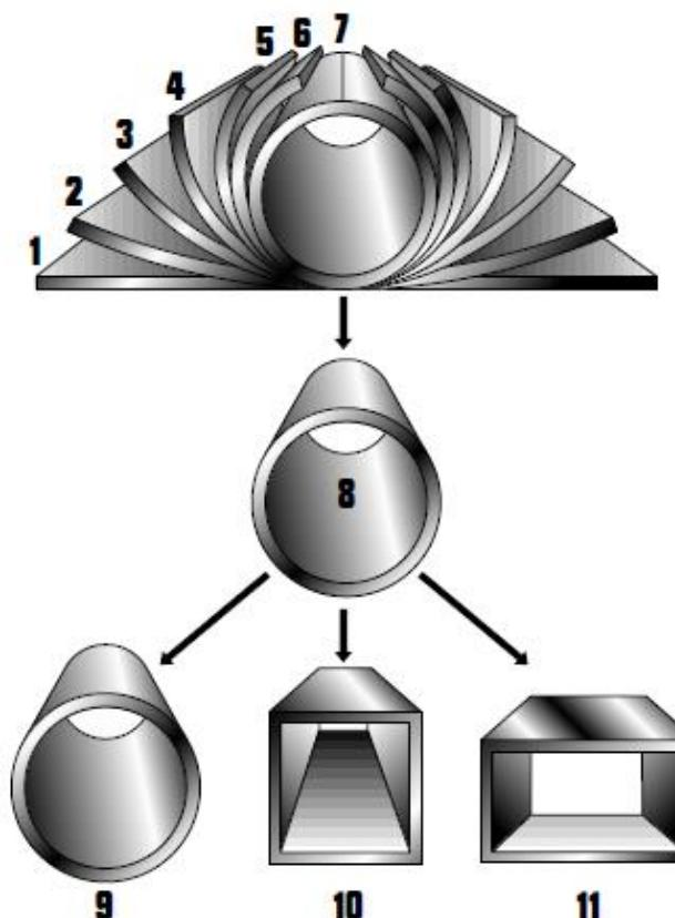
1, Electric Resistance Welding Process
