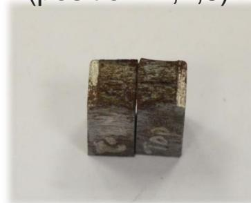
Specimens from the hot-formed hollow section (position: 1,2,3)
