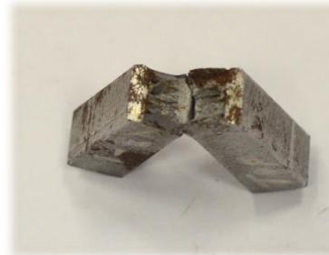
Specimens from the cold-formed hollow section (position: 1,2,3)
