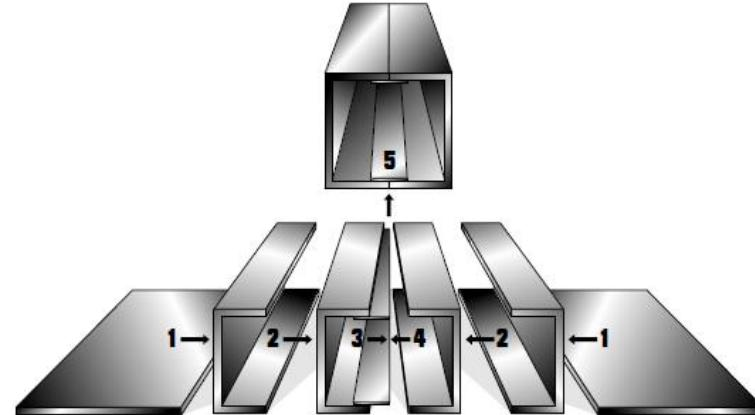
3, Submerged Arc Weld Process
