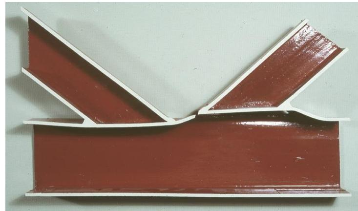
Plastification failure – Formation of Plastic Hinge at Weld Toe
