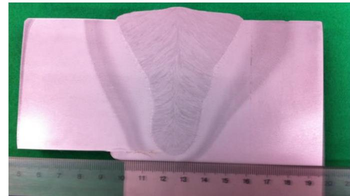
HAZ by high heat input SAW
